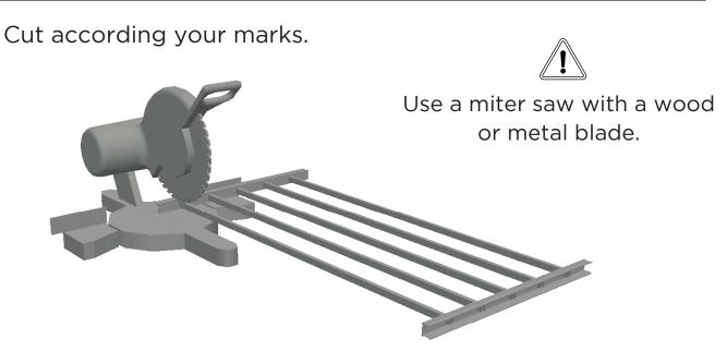
Cut the finishing trims 1/16" less than your "L" measurement from step 1. This is to avoid scratching door jambs during installation.
