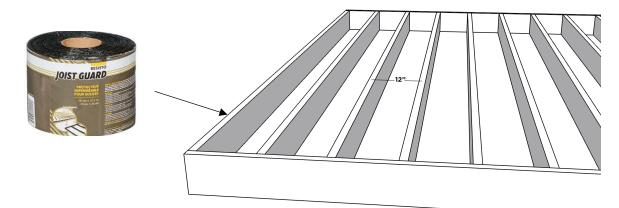
Once deck boards are installed, they must exceed of 1" to 1,5" min. from structure and its finish (fascia, vertical boards, etc.). Before building the structure, it's important to evaluate this overflow. That means if you want a 10' x 16' final size-deck, the structure must be a little bit smaller.
