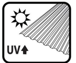
**Note: Exterior side of the panel (the one with UV protection) should have the corrugations pointing down on the sides (like an m).**
